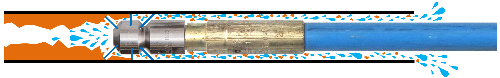
Heavy scale, nozzle can not pass the tube – not fully clogged
