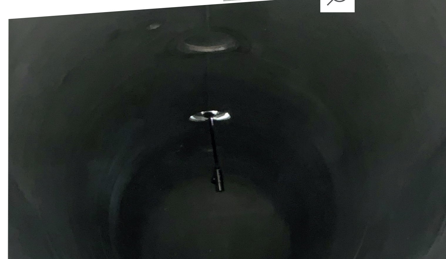
Set into rotation by recoil force of water jet
