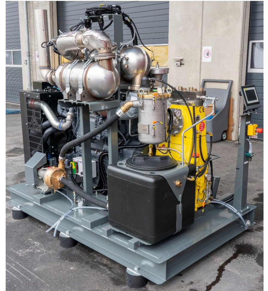
Aquajet® 14 stationary 22l/min @ 3200bar | Tier-V Deutz engine
